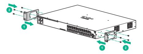
**2.** Use rack screws to secure the brackets to the rack.
