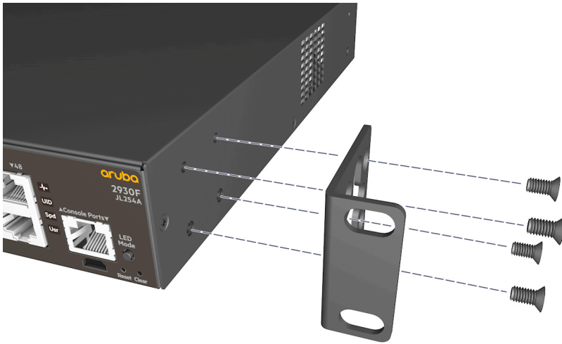
Figure 8: Attaching mounting brackets to the 2930F 24- and 48-port switches
