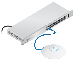
UniFi Switch Power Connection Diagram
